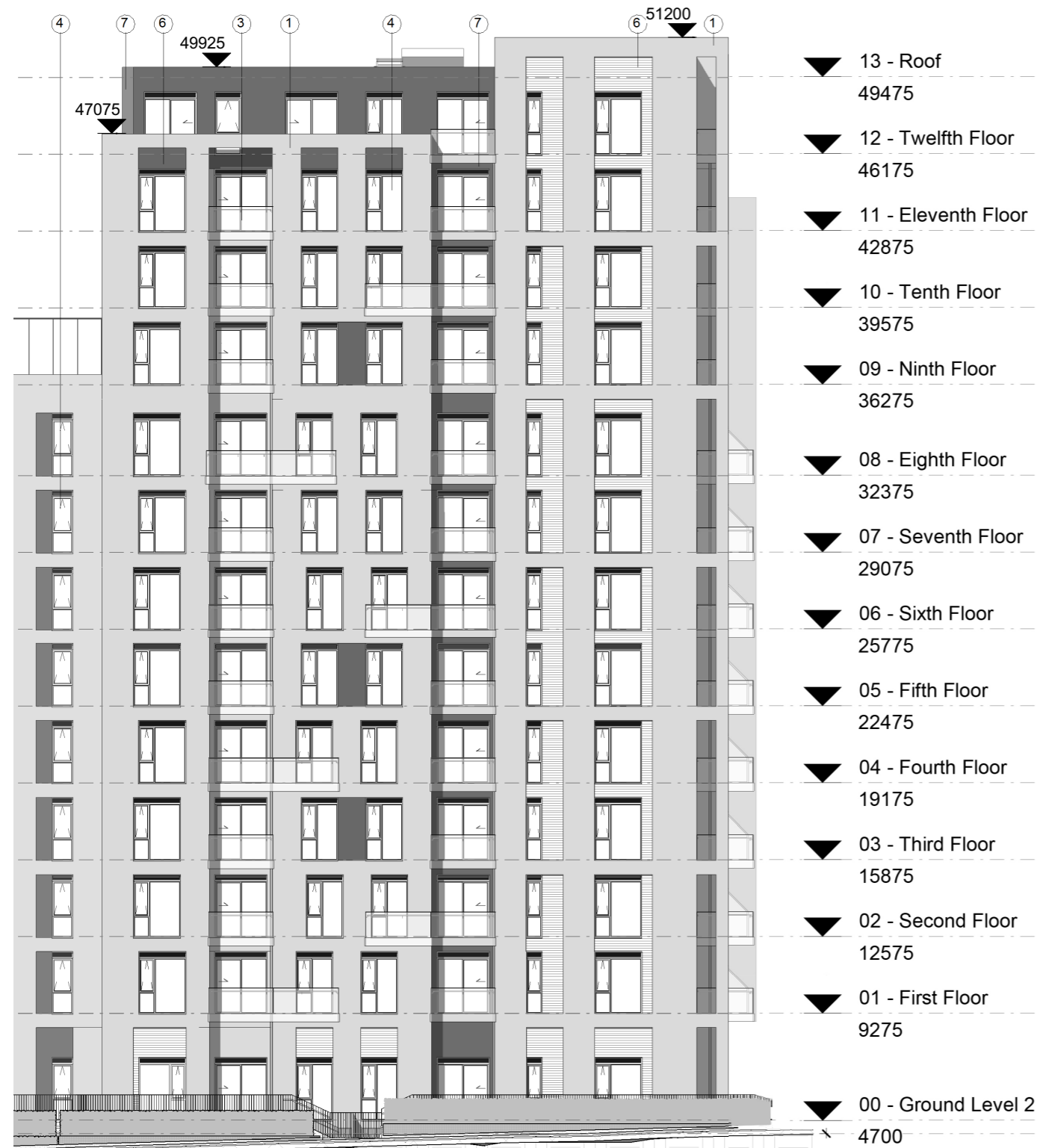
Floor to Ceiling Heights - North Elevation
